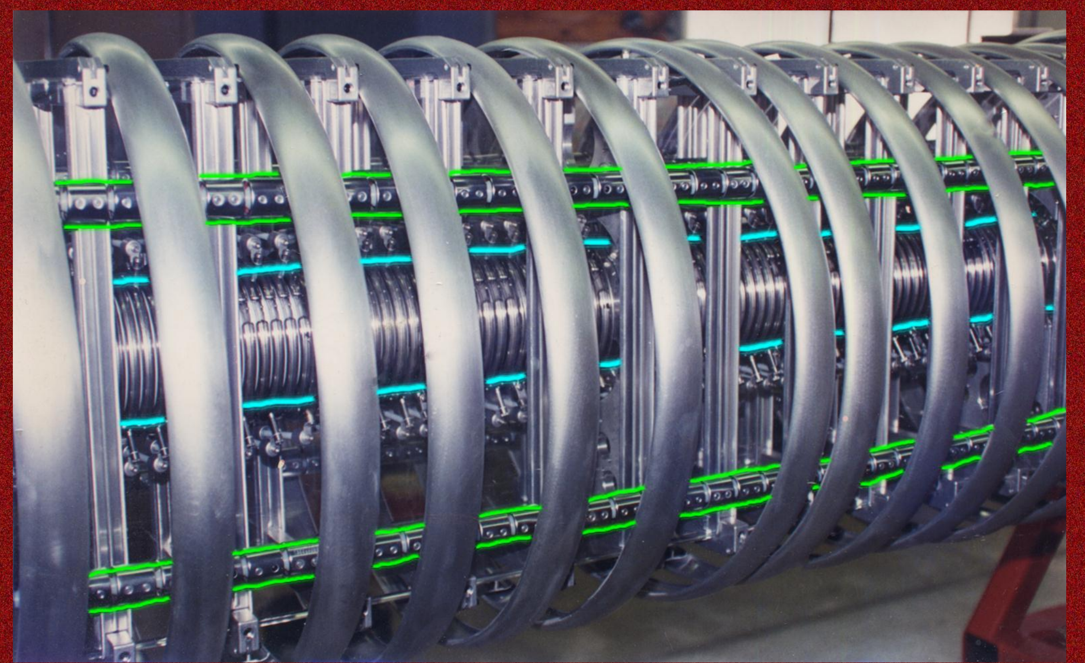
The gradient rings maintain a uniform potential. The chain (green) carries charge to the dome. The beam is accelerated through the inner tube (blue).
